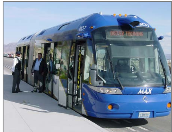
Figure 41: An example of a bus rapid transit vehicle, which is designed to look and function similar to a light rail vehicle.
